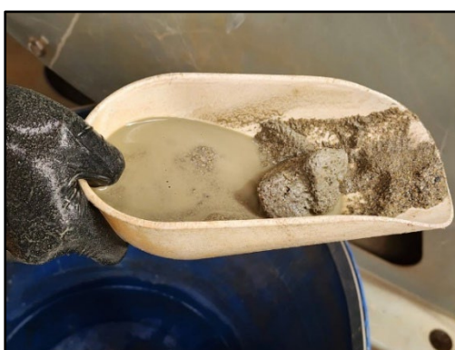
Figure 6: Sample taken directly from the scrubber showing coarser and fine, sand-like particles.
