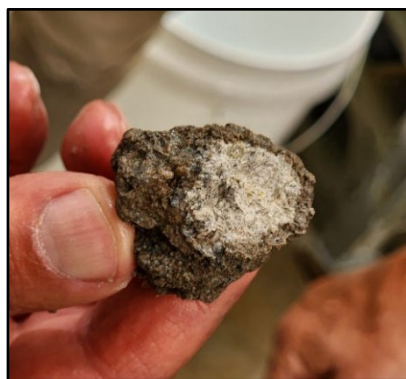
Figure 5: Fractured and partially wetted sample.
