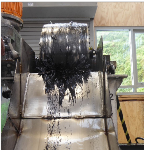
Magnetite concentrate on Low Intensity Magnets (LIMS)
