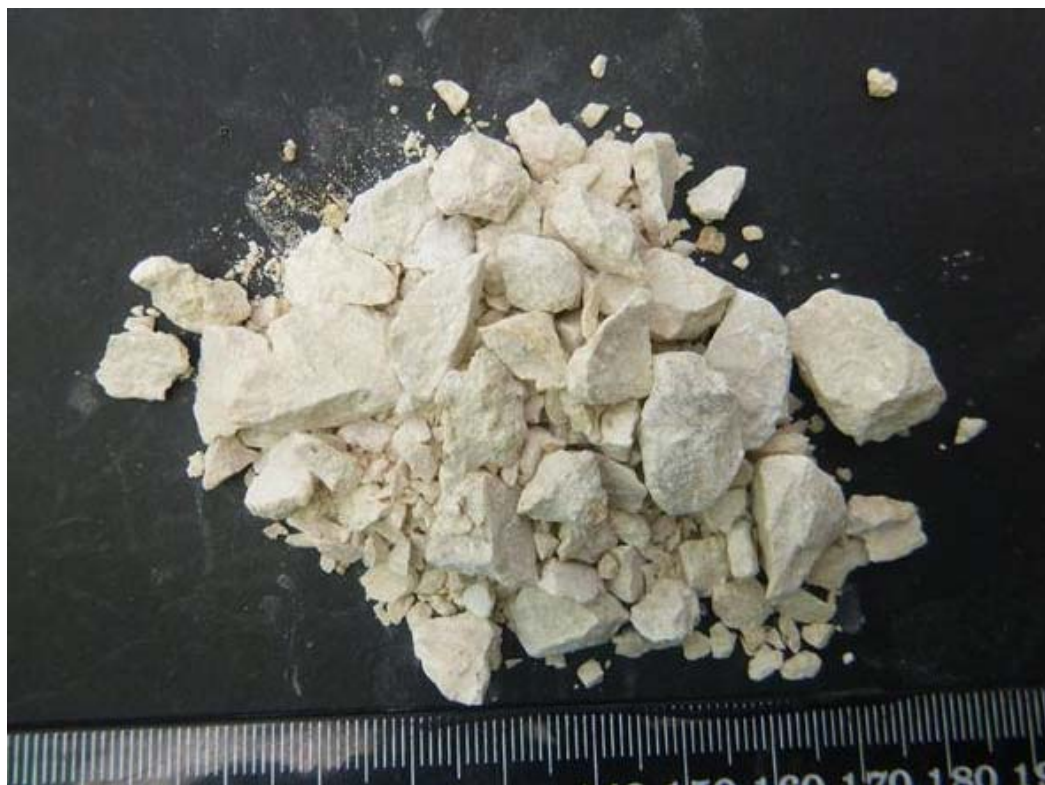
Figure 6 - limestone was crushed for petrography analysis, and shows good aggregate potential and shape
