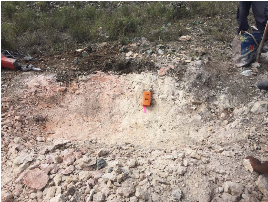
Figure 3 – Limestone sample pit at Kido deposit showing the limited thickness of overburden occurring on site.
