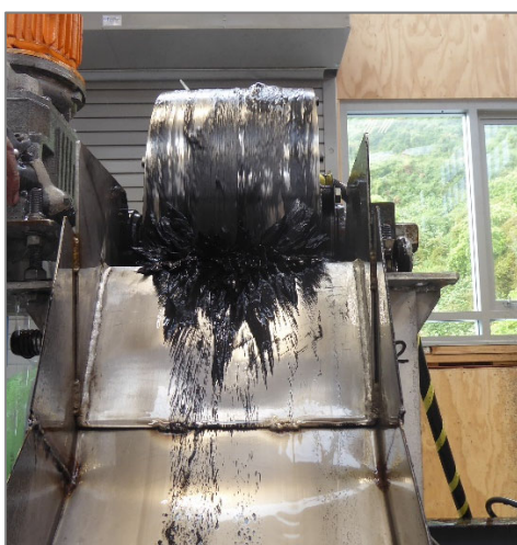
Magnetite concentrate on Low Intensity Magnets (LIMS)
