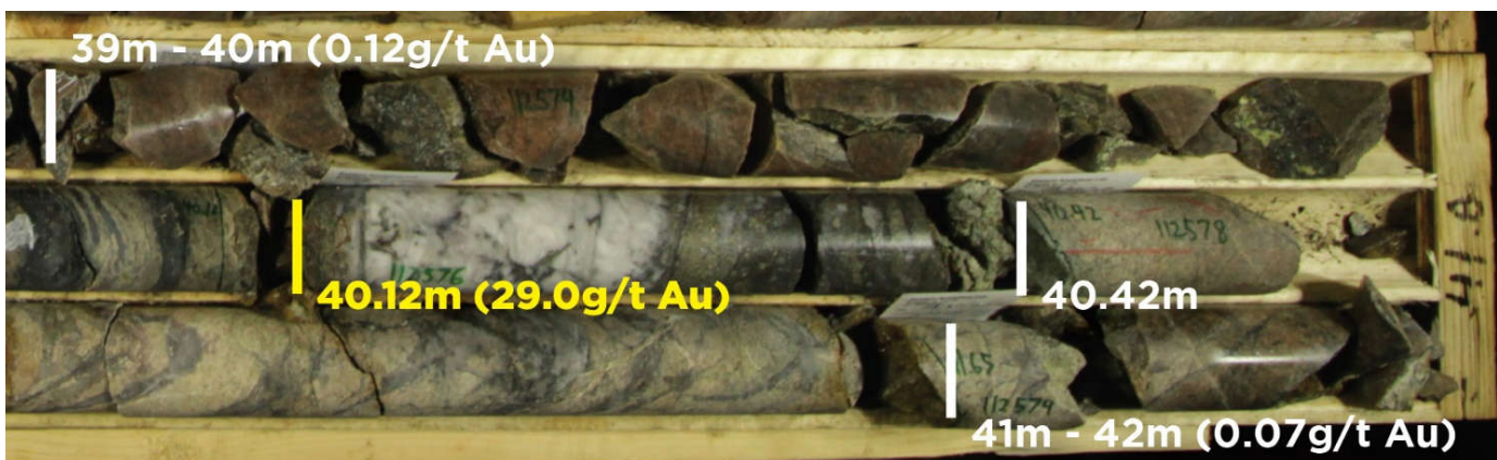
Figure 5: Quartz-galena vein mineralisation typical of WGH in hole CRD130 (40.12 to 40.42 metres) including interpreted subordinate stockwork vein array (40.42 to 41metres)
