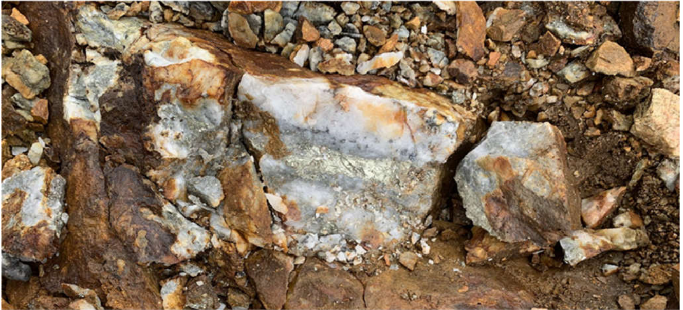
Figure 7: Example of an outcropping, steeply south-east dipping, laminated quartz-galena-pyrite-chalcocopyrite vein south-west of the WGH Resource
