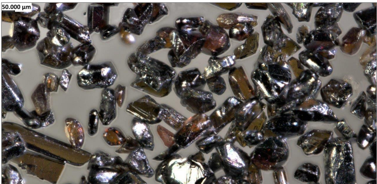
Figure 9: Photomicrograph of high purity rutile product 97.2% TiO 2 .
