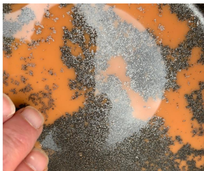
Figures 11 & 12: Very coarse-flake graphite in +600µm sample fraction (L), graphite floating on soaking drill sample (R).
