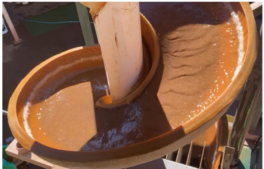
Figure 7 & 8. Left: Gravity spirals set-up for the processing of the deslimed and screen material & Right: Close-up of the gravity spiral in the early phases of the process
