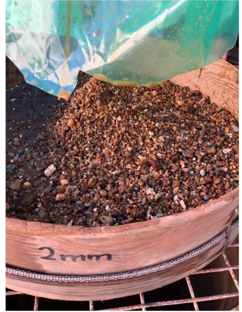
Figure 5 & 6. Left: Trommel screen processing the raw material & Right: +2mm oversize material
