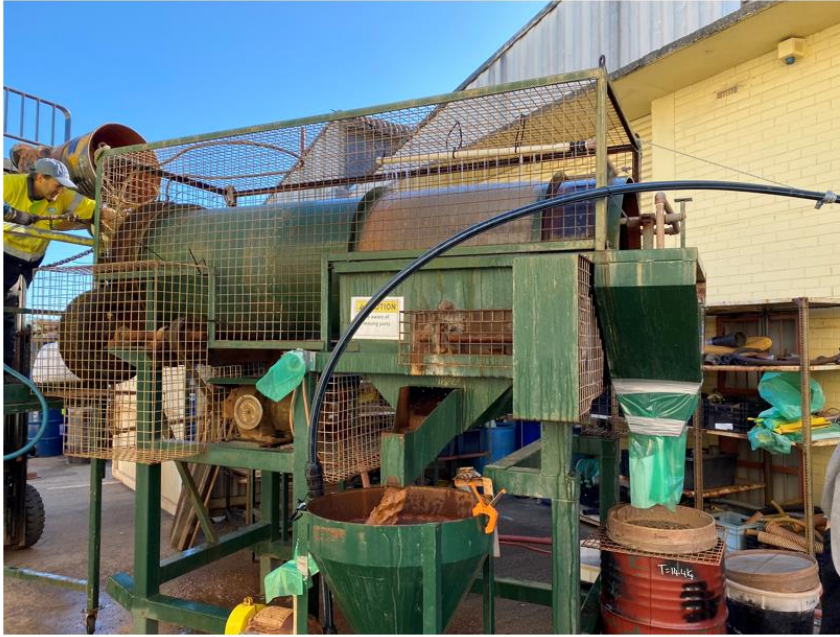
Figure 5 & 6. Left: Trommel screen processing the raw material & Right: +2mm oversize material
