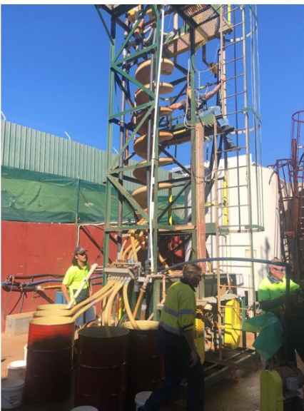
Figure 7 & 8. Left: Gravity spirals set-up for the processing of the deslimed and screen material & Right: Close-up of the gravity spiral in the early phases of the process
