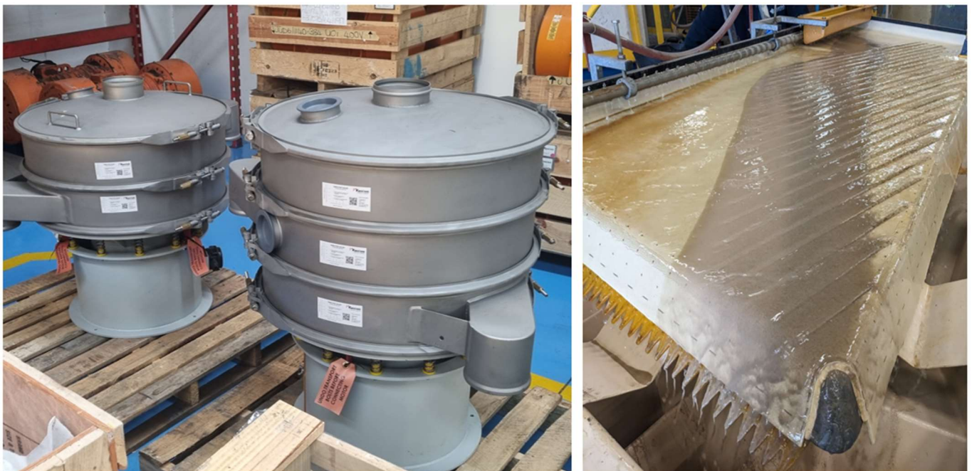
Figures 5 & 6: LHS: Kwatani shaking screens prepared for despatch to Malawi. RHS: An example of the Holman-Wilfley 2000 Series shaking table that has been ordered and is currently under fabrication
