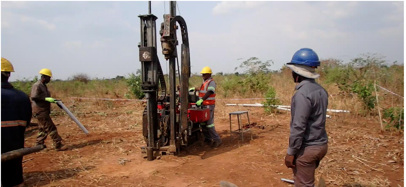
Figure 3. Push-tube core drilling at Kasiya.
