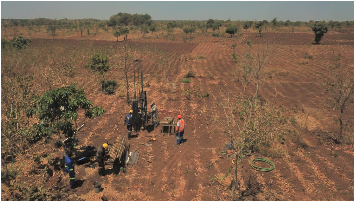
Figure 4: Drone photograph of the push-tube core rig in action at Kasiya.
