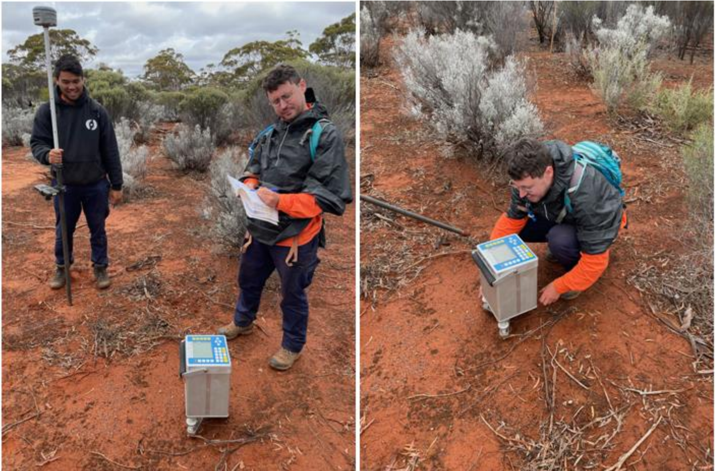
Figure 2: Technicians taking gravity readings at Hickory.
