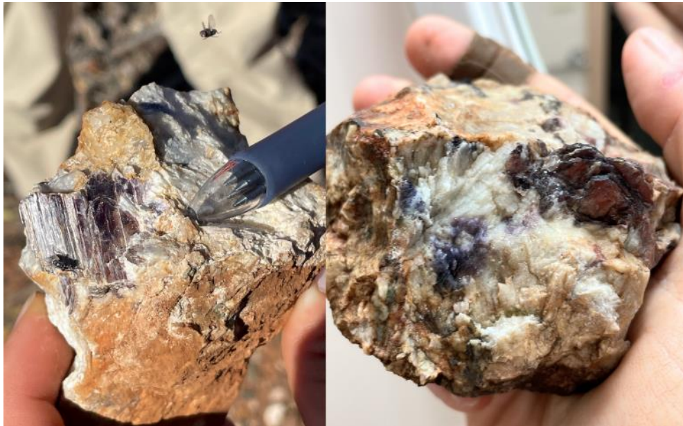
Figure 6: Rock chip PN002 showing coarse lepidolite crystals in pegmatite with assay of 0.16% Li 2 O
