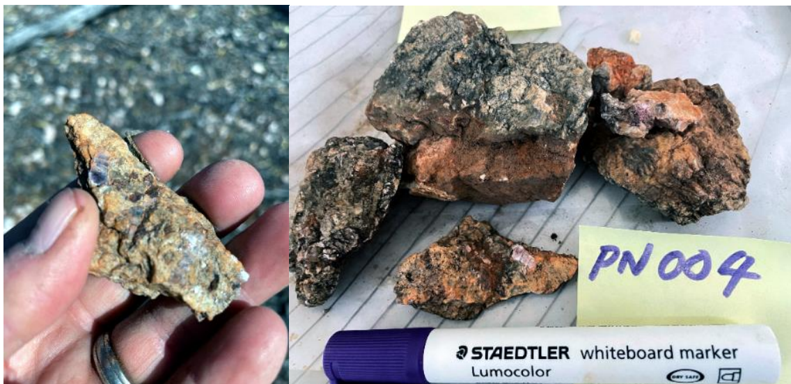
Figure 7: Rock chip PN004 showing coarse lepidolite crystals in pegmatite which returned 0.45% Li 2 O
