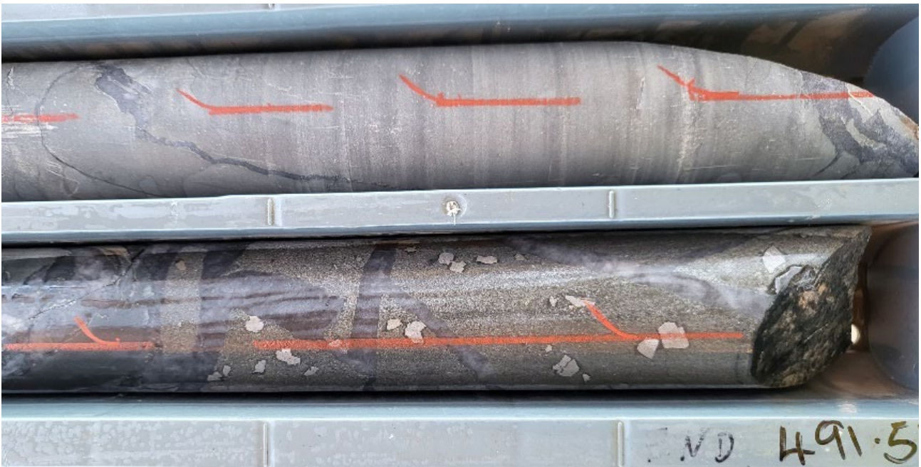
Figure 4: Core photo of 22CYDD007A showing arsenopyrite from an ~8m interval. Assays results are 4.46m @ 7.71g/t Au from 496.84m (including 0.71m @ 20.20g/t Au from 497.64m)
