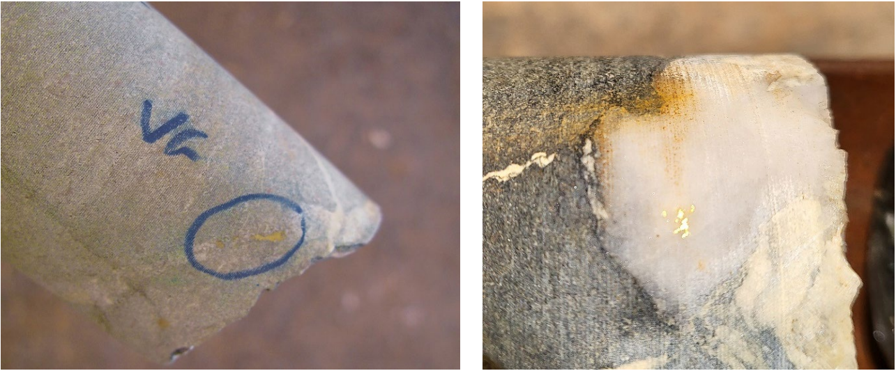
Figure 7: Core photo of 22PGRD019 (left) at ~115m depth and 22PGRD010 (right) at ~49m depth showing visible gold in a quartz vein within the Paulsens Mine Gabbro. Assays are for this hole are expected in December 2022.
