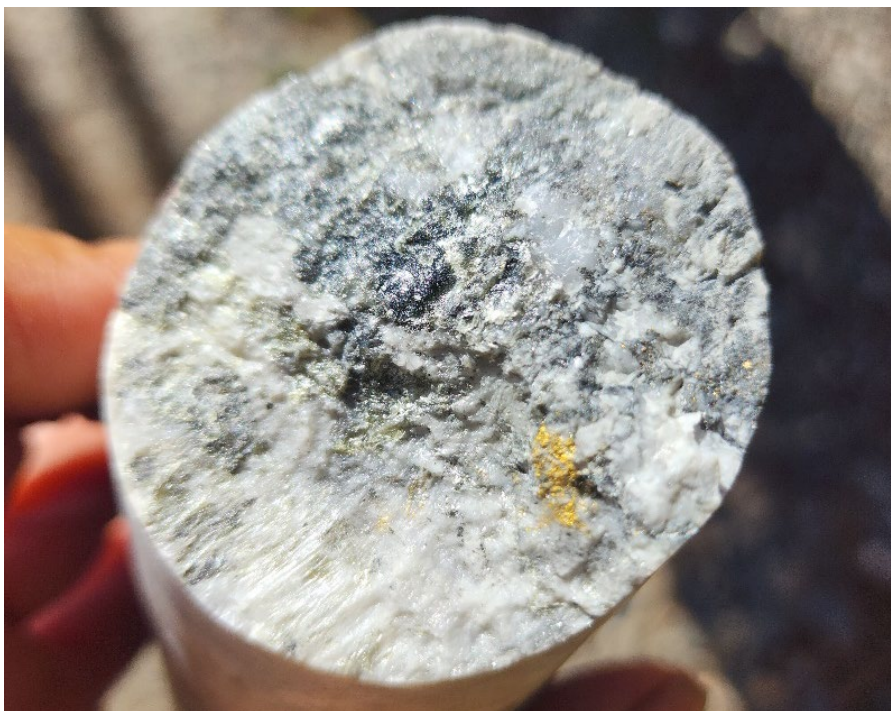
Figure 1: Visible Gold in PGRD23002 (65m depth). This interval returned 0.56m @ 35.30g/t Au from 64.87m
