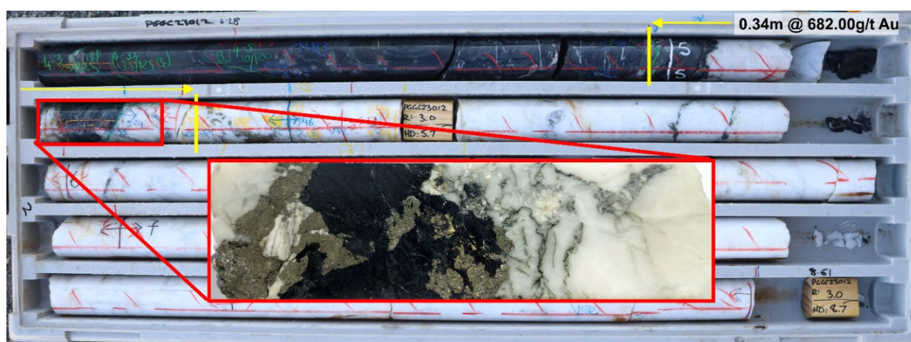
Figure 1: Core photo of PGGC23012 showing the 0.34m @ 682.00g/t interval with abundant visible gold.
