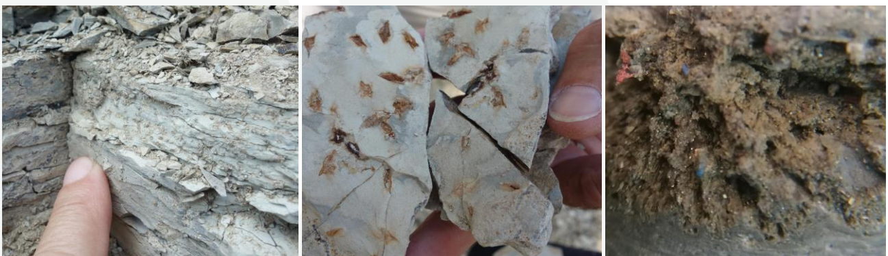
Figure 1 - Disseminated nodular analcime (left) and oxidized sulphide lenses (middle), and fine, disseminated sulphides replacing most likely soluble borate minerals - pseudomorphs (right)
