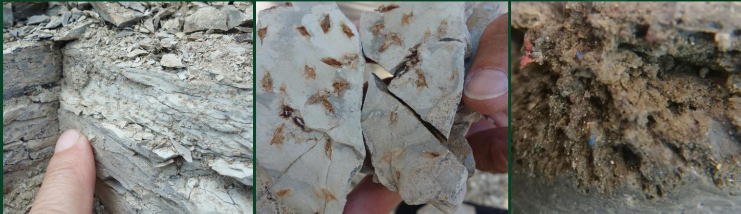
Disseminated nodular analcime (left) and oxidized sulphide lenses (middle), and fine, disseminated sulphides replacing most likely soluble borate minerals – pseudomorphs (right)
