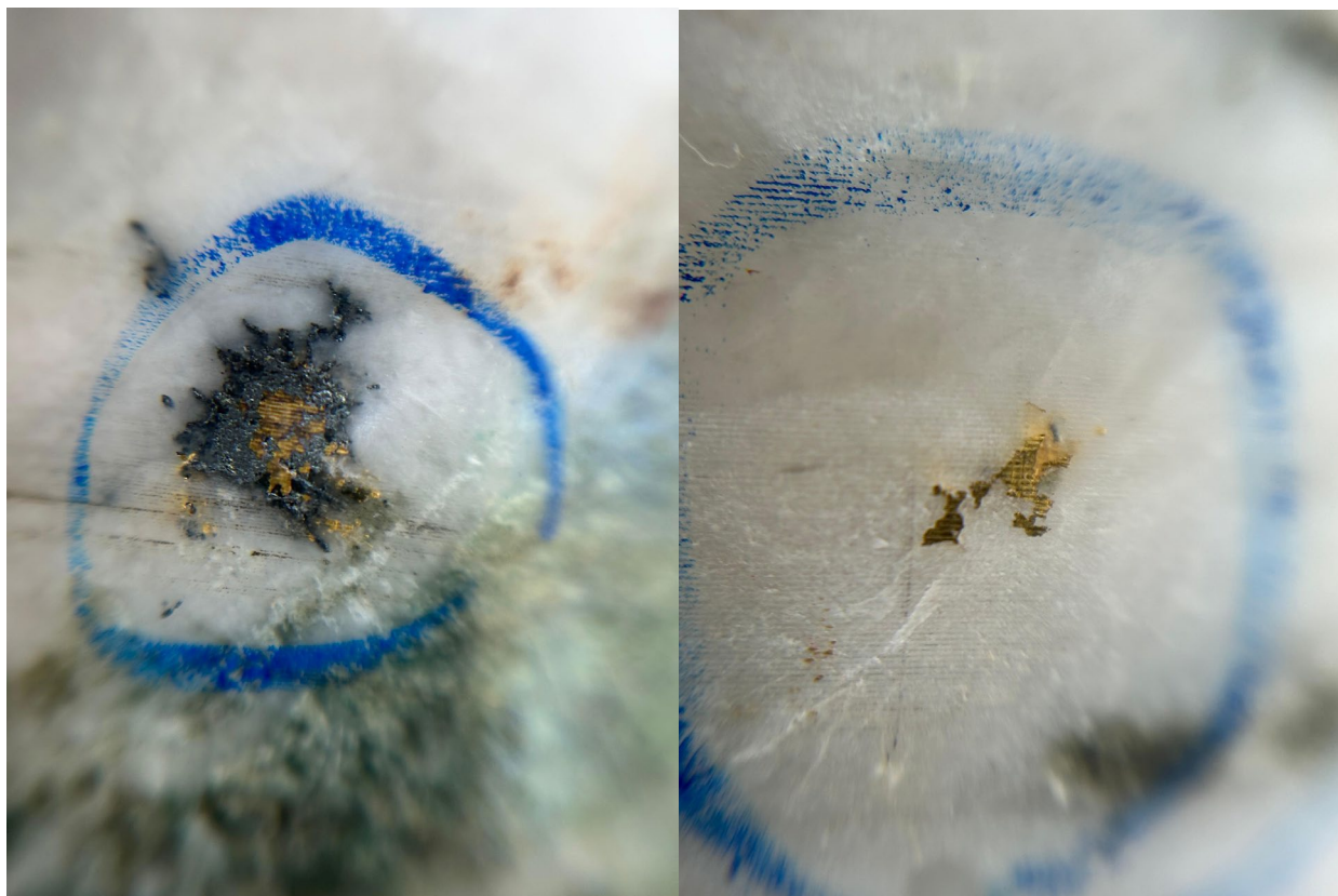
Figure 5: Close up visible gold in 24BTDD002. Close association with galena visible (left), free gold (right)
