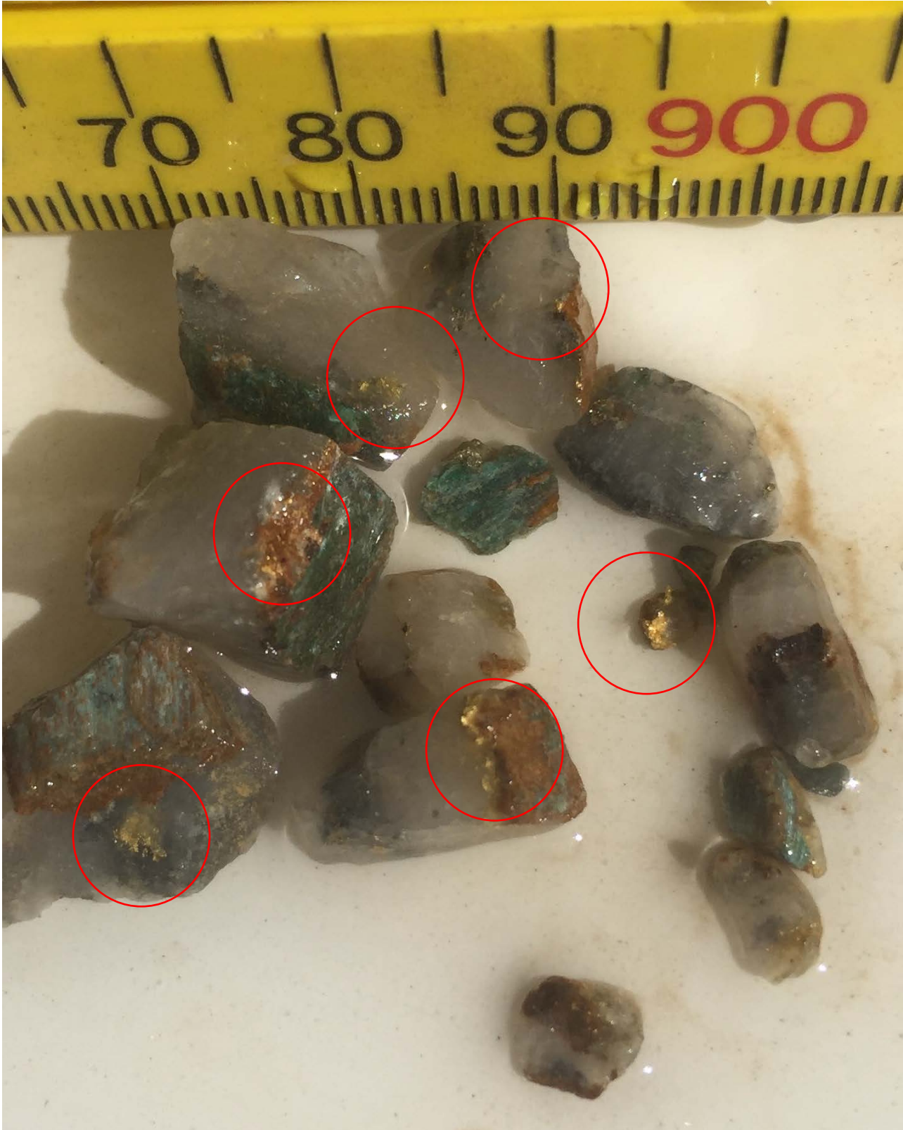
Figure 3: RC Chips from 17KLRC032 showing Visible Gold (significant intercept of 6m @63.31gt, including 2m@182.57g/t reported ASX Aug 21)
