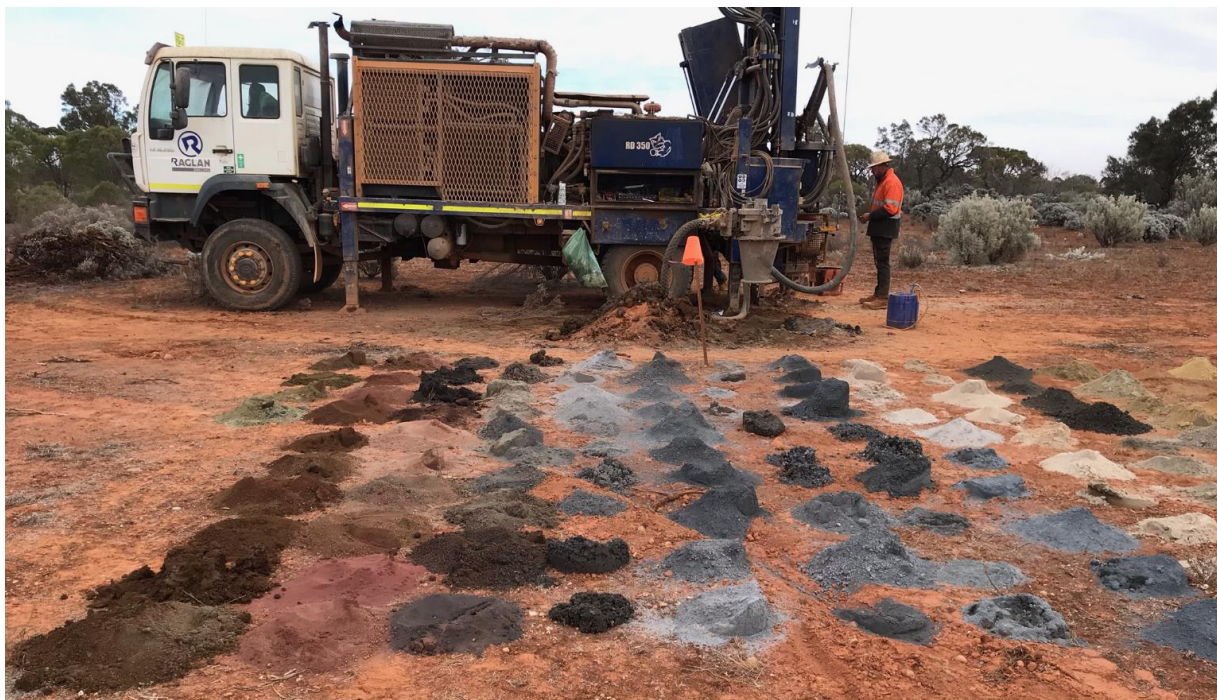
Figure 6: Air-core drill samples in the Fraser Range.
