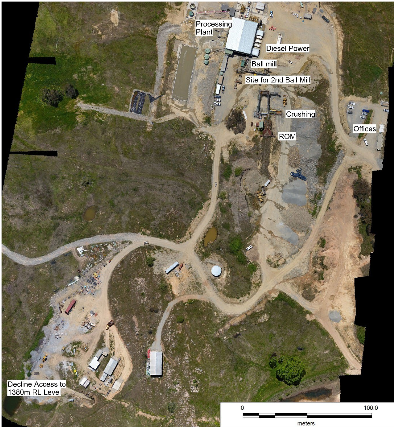
Figure 2 Mine Site Aerial View generated from a Drone Survey that shows the location of the Decline to the Underground 1380mRL Level and location of ROM Stockpiles
