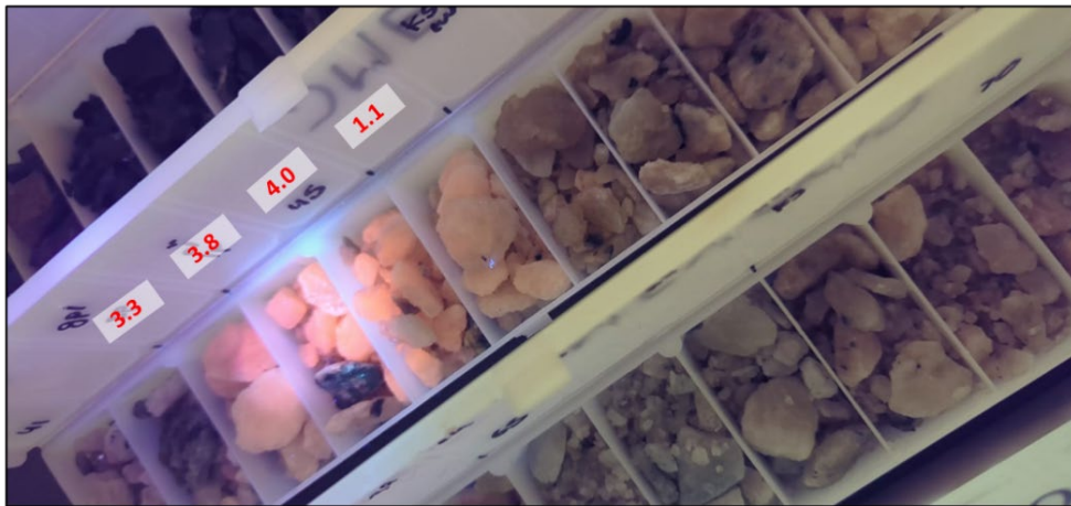
Figure 3: Photo of pegmatite bearing portion of JREX002 with spodumene fluorescing under UV spot torch with Li 2 O % grades above the fluorescing intervals. The assay results received for this hole confirm the
