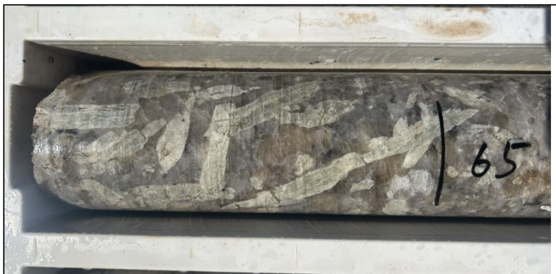
Image 2: KHDD001 showing of coarse spodumene in drill core at 64.9-65.1m down hole depth (pale green elongated phenocrysts) – awaiting assays
