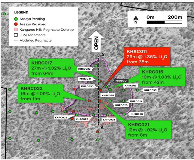
Figure 1: KHLP - Drill Holes Plan View
