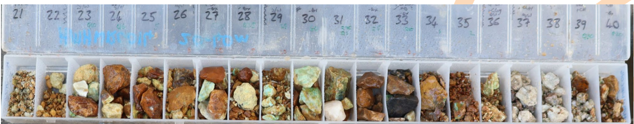
Figure 1. Copper oxide visible in drill chips from HMHWRC0014 (20-40m). A copper grade of 2.78% was reported between 31m and 36m (see ASX Announcement 31 October 2023).
