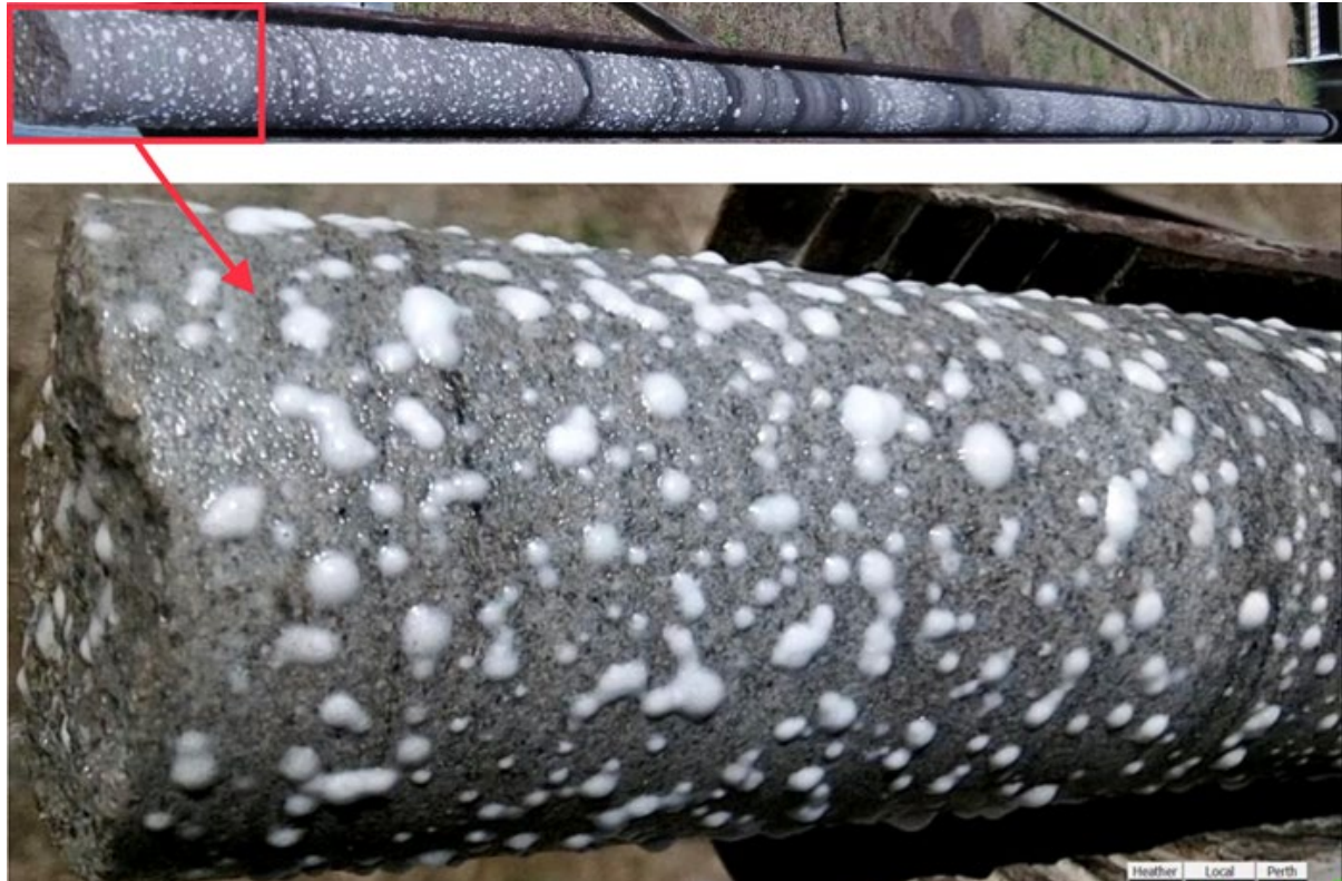
Figure 2- Visible gas emissions from core samples from 270-06C
