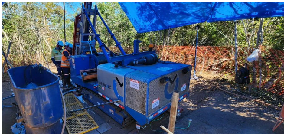
Figure 1: Large diameter core drilling rig on site at Colina
