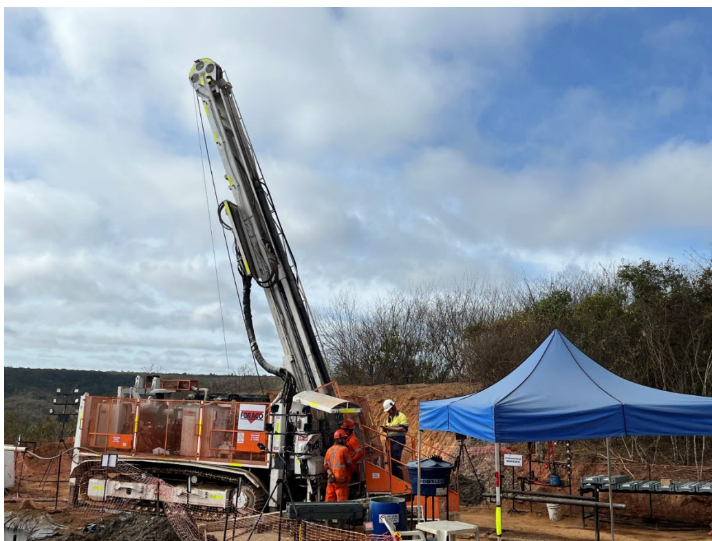
Figure 7: CS3001 drill rig, one of the two metallurgical drill rigs currently on site, drilling SAMT002.
