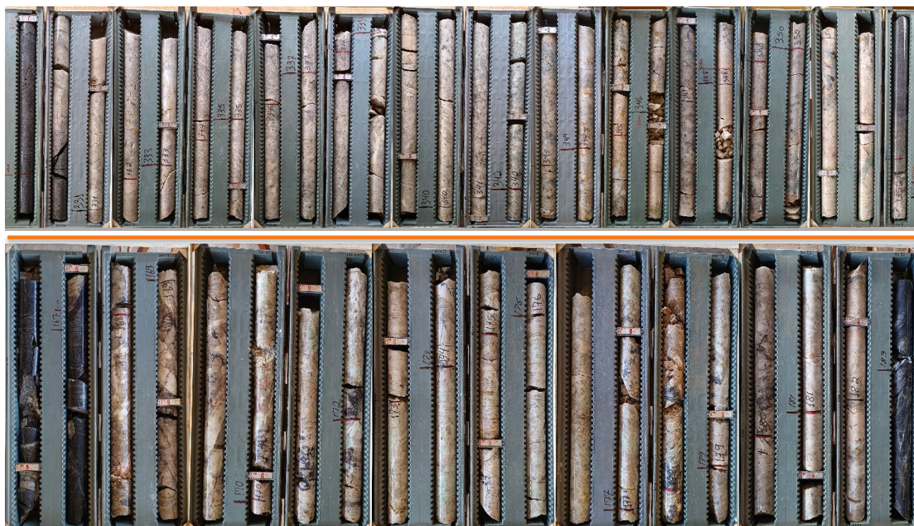
Figure 6: Diamond drill core showing spodumene minerals for SAMT001 (top) at intervals 330.25 to 352.20m; and SAMT002 (bottom) at intervals 167.07 to 182.5m. Refer to Appendix 4 for further details.
