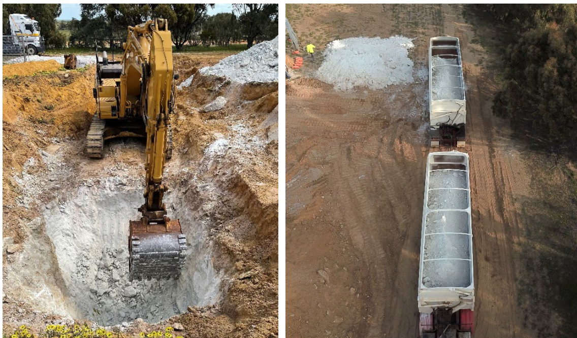
Figure 7: Further test-pit progress photos showing kaolin product to be shipped out to potential customers
