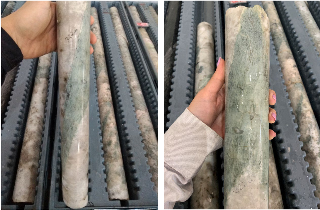
Figure 3: SADD033 – Spodumene rich pegmatite over 18.75m down hole thickness (321.15-339.90m)
