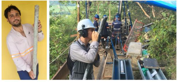
Figure 2: Bananal Valley Project – Latin Resources Senior Geologist with spodumene rich pegmatite core, and core logging on site
