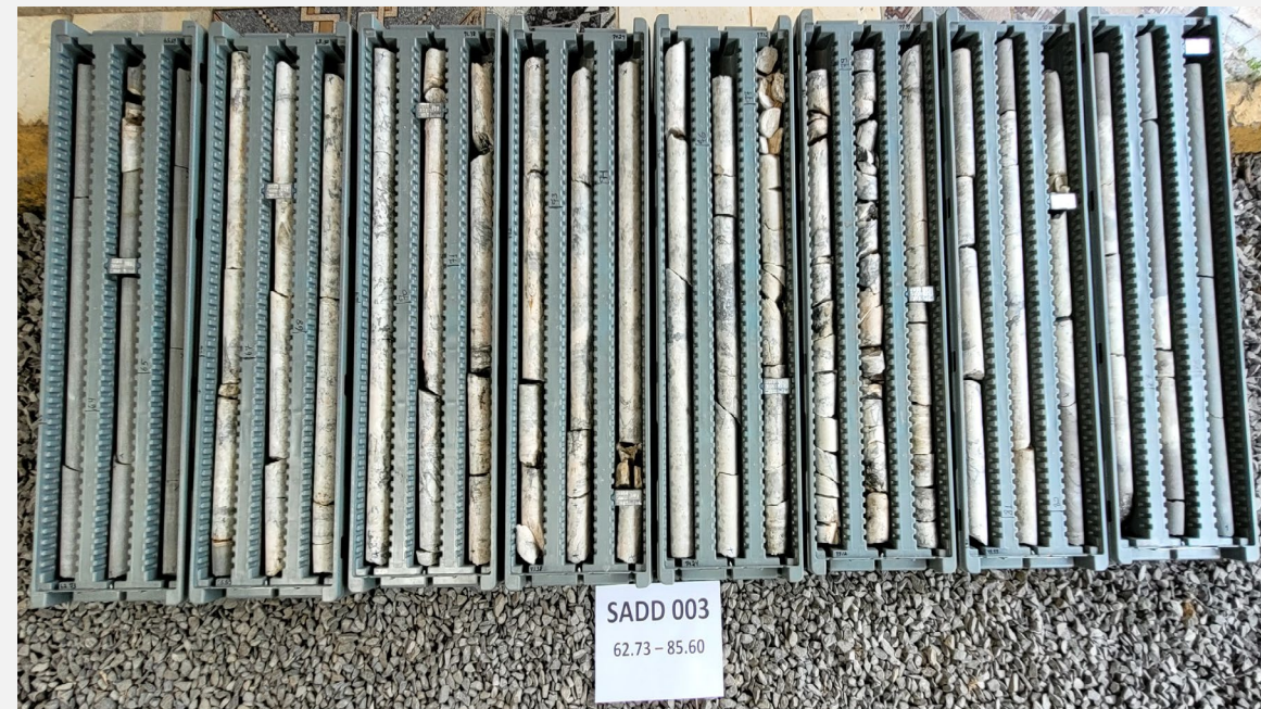
Drillhole SADD003 – spodumene bearing pegmatite 65.6-81.77m, (16.17m true thickness) intersected in diamond drilling approximately 180m along strike to the south of previously reported intersections
