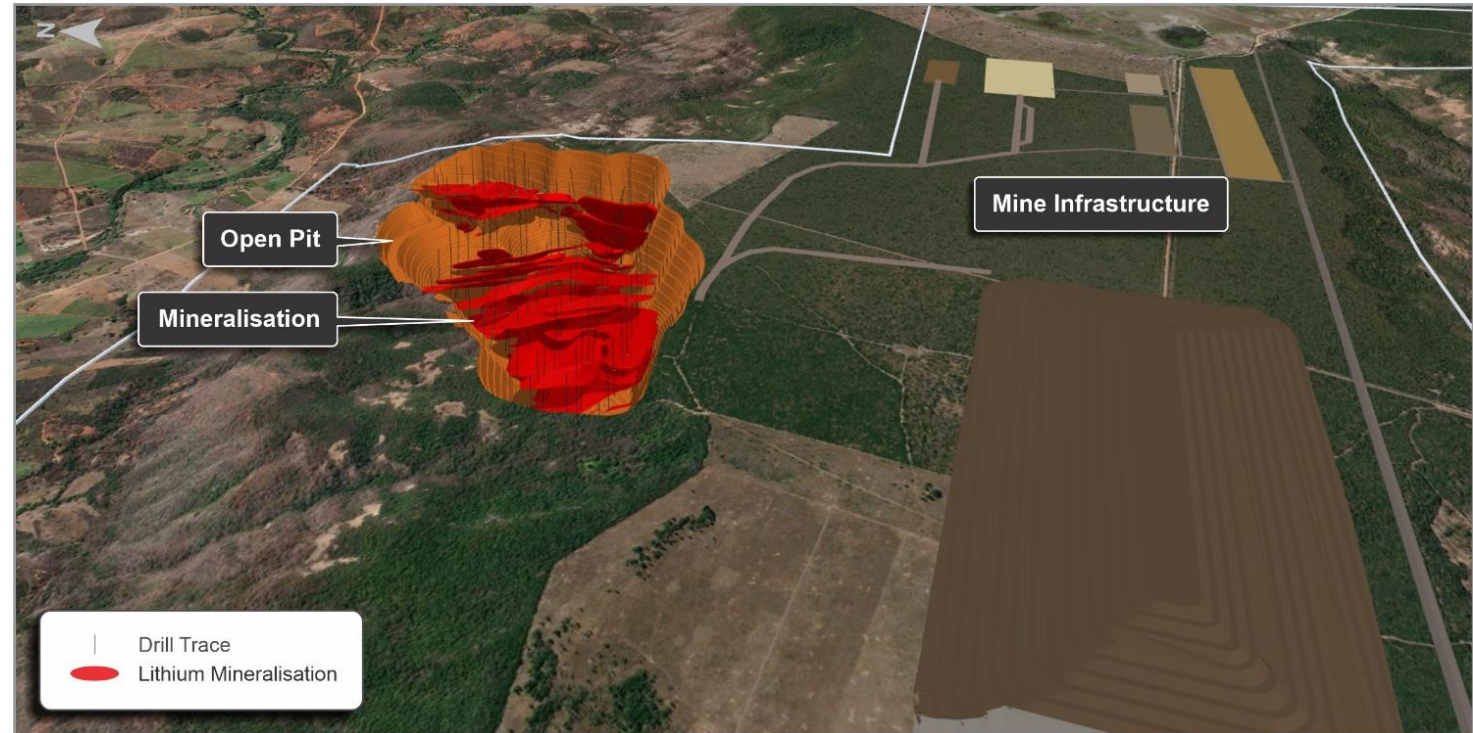
Figure: Oblique 3D view of the proposed Colina Project open pit mine (looking NE) with mineralisation and infrastructure.
