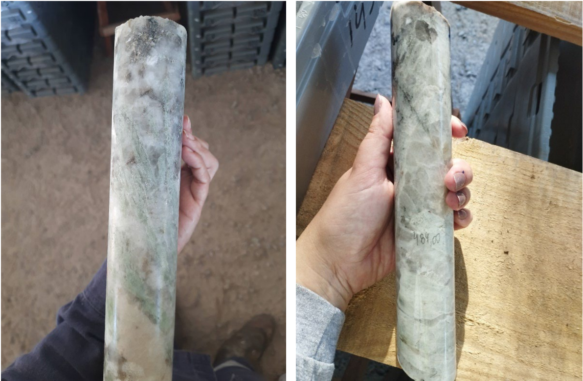
Figure 3: SADD132 (left) and SADD137 (right) DD core showing spodumene mineralisation at 394.0m and 484.0m respectively. The Company draws attention to uncertainty in reporting visual results. Visual estimates of mineral abundance should never be considered a proxy or substitute for laboratory analyses where concentrations or grades are the factor of principal economic interest. Visual estimates also potentially provide no information regarding impurities or deleterious physical properties relevant to valuations. Assay results are expected to be available in approximately 4 weeks.
