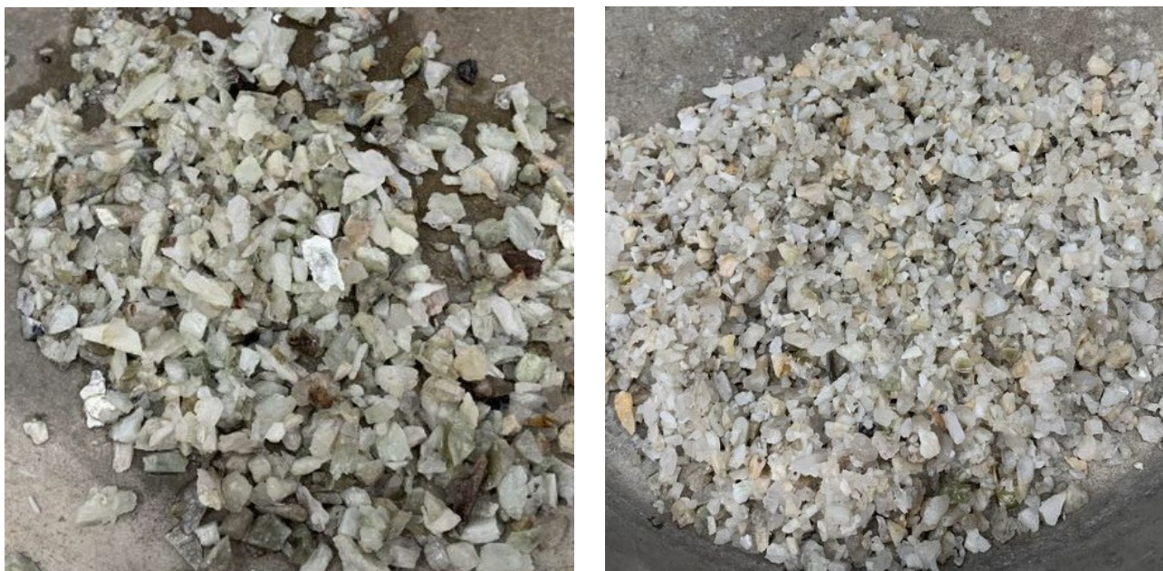
Figure 7: Colina composite 1 indicating 6.3mm (+1mm) sink (left) and float (right) results produced from DMS test work on the Colina ore samples.
