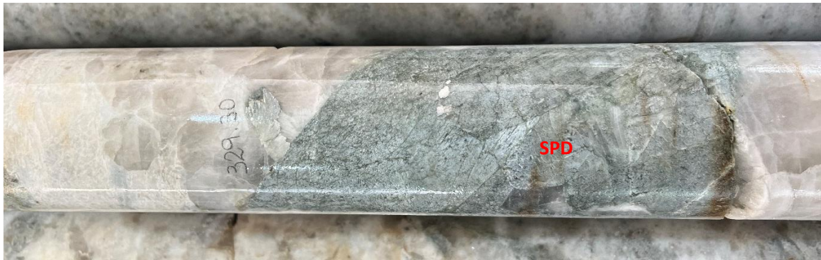
SADD246: ~329.30m (1.78% Li 2 O). Green spodumene associated to quartz, feldspar and mica
