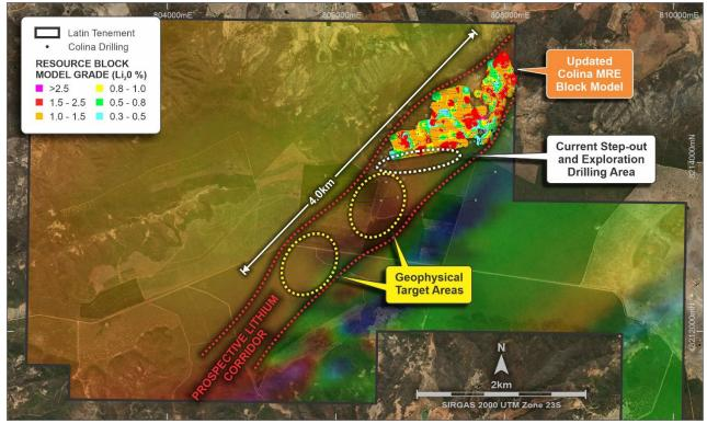
Figure 5: Colina Deposit MRE area, highlighting the interpreted prospective Li corridor and newly identified geophysical<sup>3</sup> drilling target areas
