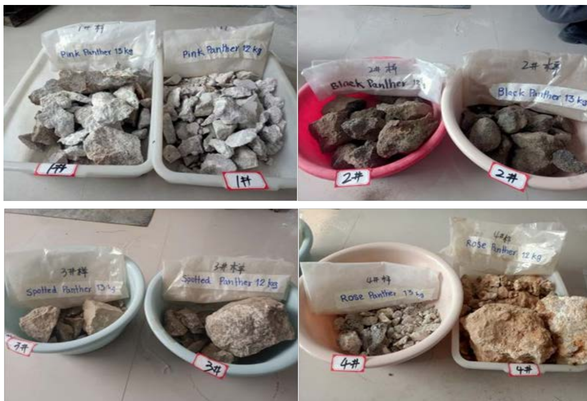
Photo set 2 - (testwork samples - from left to right and top to bottom) lepidolite sample from Pink Panther, polyolithionite sample from Black Panther, polyolithionite sample from Spotted Panther & lepidolite sample from Rose Panther
