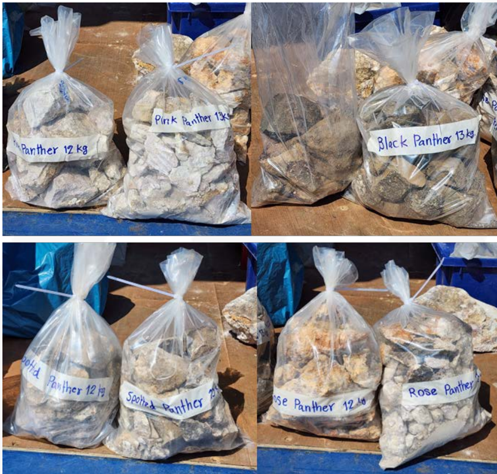
Photo set 1 - (from left to right and top to bottom) lepidolite sample from Pink Panther, polyolithionite sample from Black Panther, polyolithionite sample from Spotted Panther & lepidolite sample from Rose Panther
