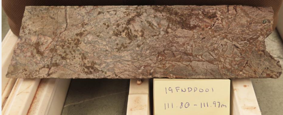
Example of basal breccia zone of the gold mineralised section - jig -saw breccia formed by seismic shock decompression and shattering of the altered country rock (has been observed in some parts of Sunrise Dam)
