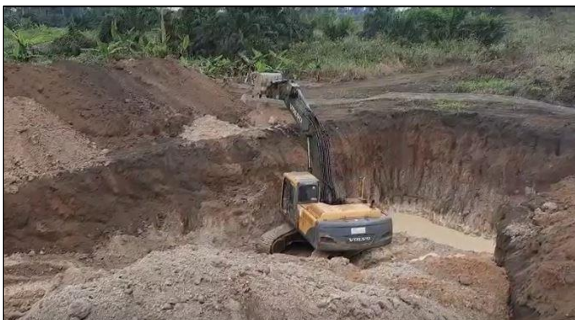
Figure 1 - Cabinda Phosphate Project, work being undertaken to complete a bulk sample.
