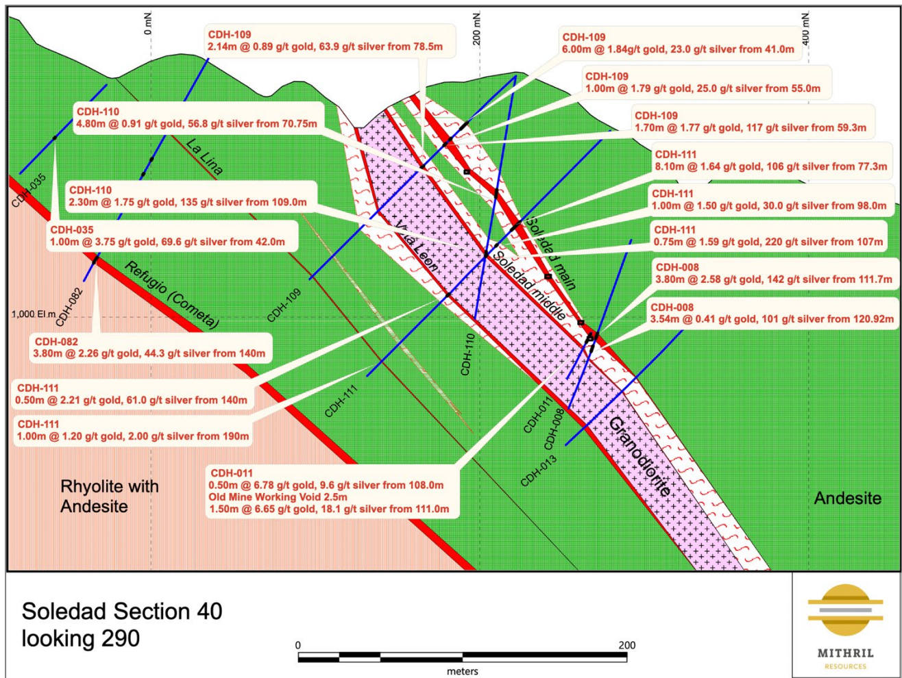
Figure 1 - Cross-section 40 for drill results at La Soledad holes CDH-109 to 111 plus previous drill hole results for holes CDH-008 and 011. Sheeted vein system associated with the granodiorite intrusion.
