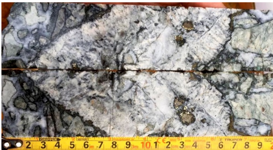
Figure 10: Two halves of cut NQ size core from hole CDH-077 472.1-472.3 metres with abundant visible gold
