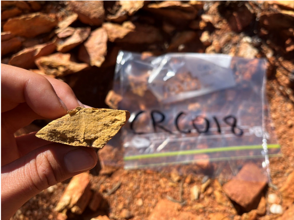
Figure 3: Silicified aphanitic kimberlite rock-chip (CRC018), 2,295ppm TREO, 150m west of peak soil sample 765ppm TREO
