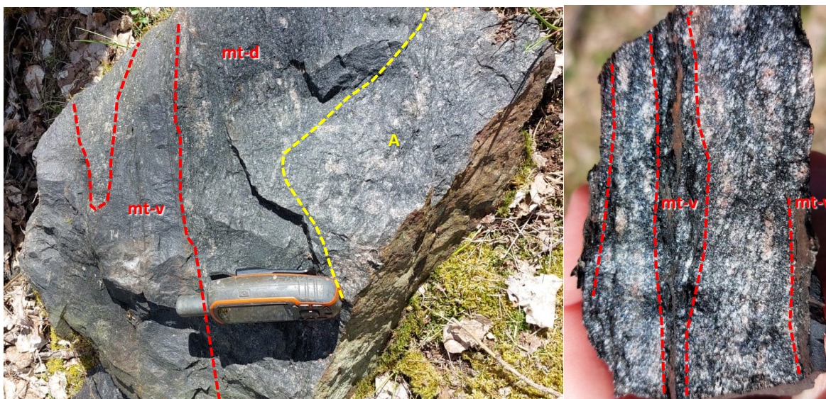
Figure 2 (left): Photograph of rock sample OLSGS003 with massive magnetite veins (mt-v) that returned 8,286 ppm TREO (86% HREE) as well as disseminated magnetite-altered (mt-d) augen gneiss (A) | (right): Photograph of rock sample OLSGS001 of biotite-altered augen gneiss with magnetite (mt-v) veins that returned 9,012 ppm TREO.
