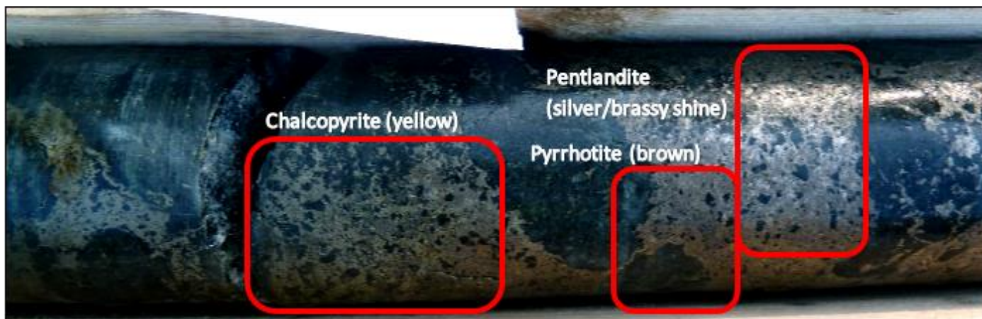
Figure 2: Close up of drill core showing Chalcopyrite (Cu), Pyrrhotite (Fe) and Pentlandite (Ni) sulphides.
