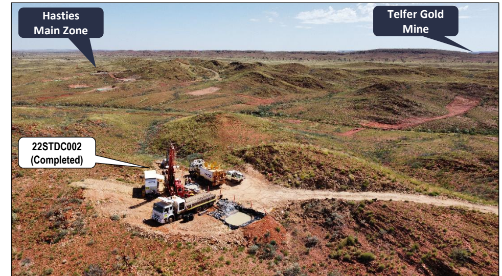
Diamond drilling to test Hasties Deep Target, ~300m SE of the Hastie Main Zone.
