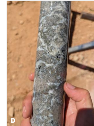
Photos: Clockwise from top left – (A) Chalcopyrite (cpy) in quartz veining. (B) Pyrite (py) ± cpy along discordant quartz-carbonate veins selvage. (C) Py ± cp veining with quartz-carbonate veining in siltstone. (D) Fine disseminated pyrite in altered and brecciated Dolerite near apex zone.
