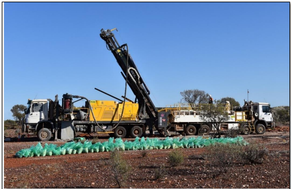
Figure 1; Orlando Drilling RC rig RC06 commencing the first hole at Mt Ida
