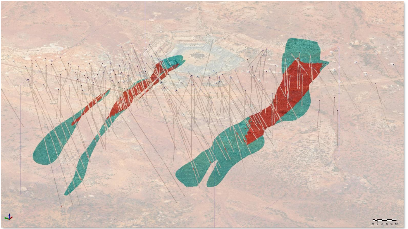
Figure 1: 3D view of drillholes and classified block models at Mt Ida with Indicated (RED) and Inferred (BLUE) Mineral Resource categories.
