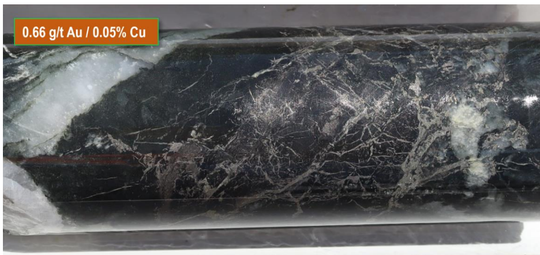
Figure 3: Mineralised Larramore core from hole 23LMDD010 (83.98-84.30m core interval) within an assayed sample length of 83.5 to 84.04 (0.54m) returning 0.66 g/t Au and 507 ppm Cu.
