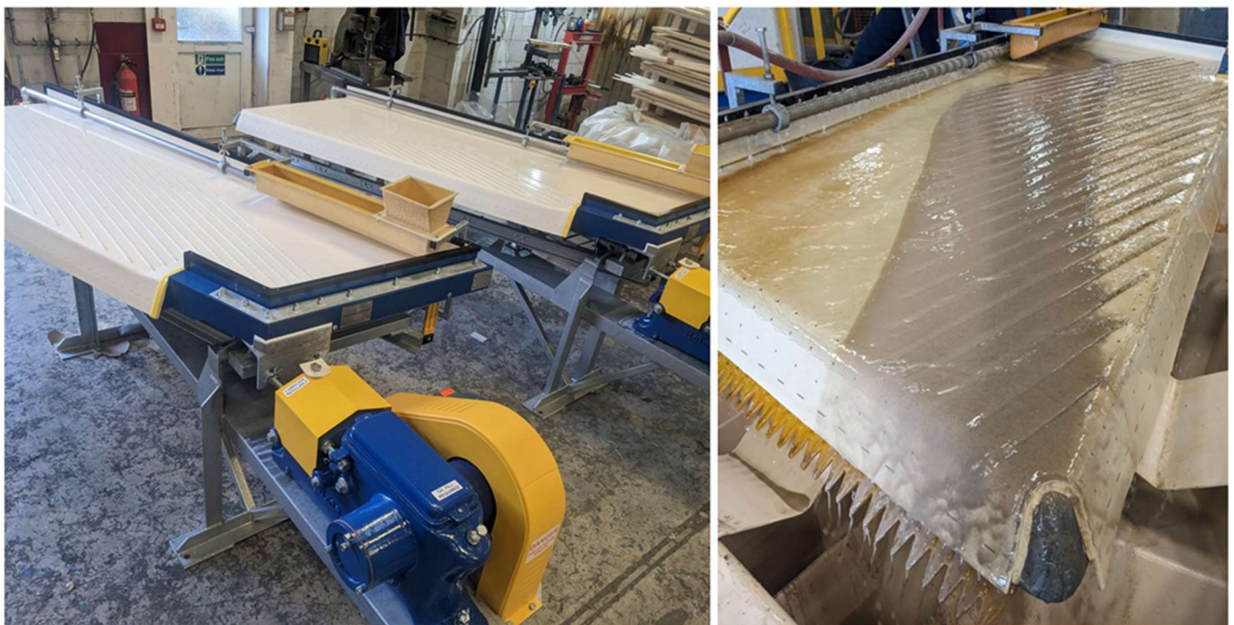
Figure 3: Holman-Wilfley 2000 Series shaking table to be installed at Sovereign's Lilongwe laboratory in Malawi.
