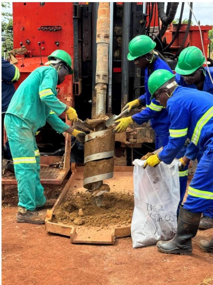
Figures 2 & 3: Bulk sample mechanised spiral drilling and sampling at Kasiya in November 2023
